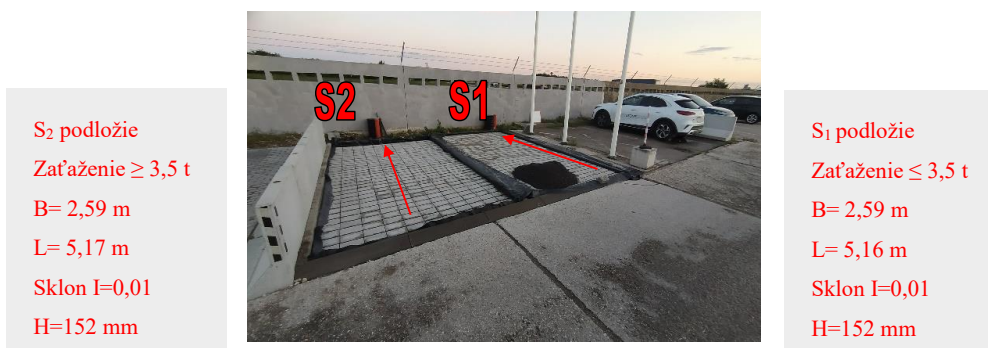
Obr. 1. Experimentálne plochy parkovísk S 1 a S 2 , zdroj NARA-SK Fig. 1. Experimental areas of parking lots S 1 and S 2 , source NARA-SK
